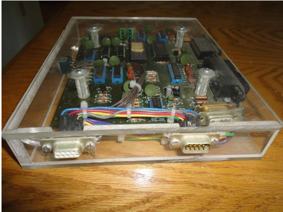
Figure 6. Front panel: 9-pin AdamNet + external-power connector (the prototype uses a 9-pin connector, not the usual RJ12).
