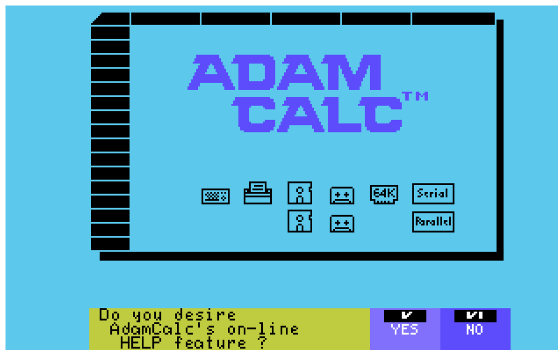
Figure. AdamCalc boot screen captured from a live emulator session after defeating the per-device AdamNet presence check at $3256 (a two-byte patch at file offset 0x0A56: B7 20 → 37 C9). All nine entries of the device-probe table at $32AB now draw their icons. The bottom row reveals the previously hidden Serial and Parallel labels.
