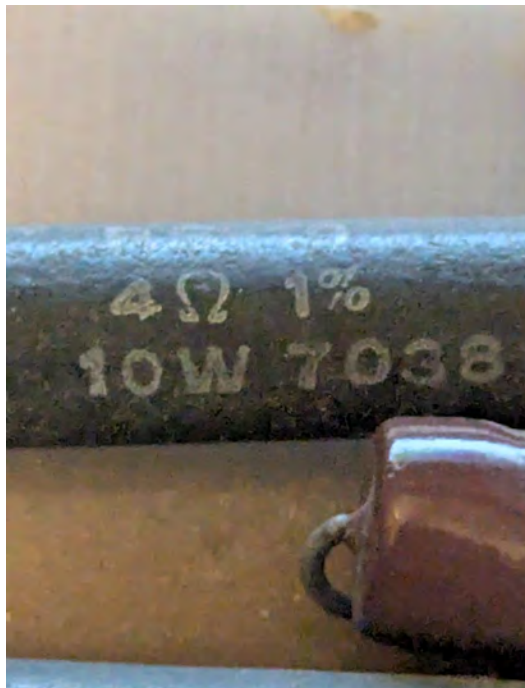
Figure 6 — R1 close-up showing the body silkscreen 4Ω 1% 10W 7038. The "7038" is a Dale internal lot/part-code suffix.
