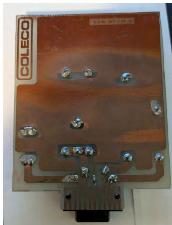
Figure 3 — Solder (bottom) side, overhead view. Single-sided FR4 construction with hand-laid copper pour. COLECO logo at upper left; foil P/N sticker at upper right (visible rotated). The edge-connector fingers at the bottom of the board fan out into hand-laid traces.
