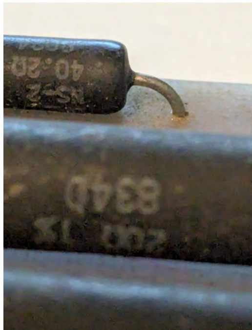
Figure 8 — R5 close-up showing 40.2 \Omega 1 % (top resistor in frame). The lower resistor shows the "8340" date code referenced for R2 (Dale week 40, 1983)
