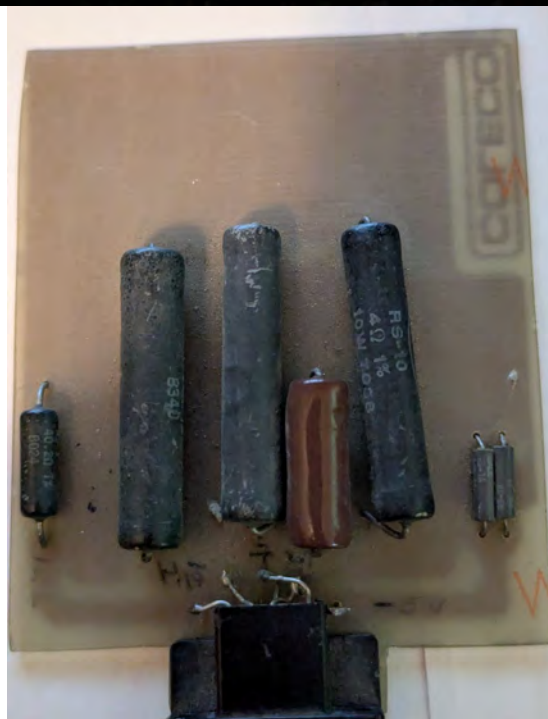
Figure 2 — Component (top) side, overhead view. Seven resistors and a single DE-9 male connector are populated on a single-sided FR4 board. The faded COLECO logo is visible at upper right.
