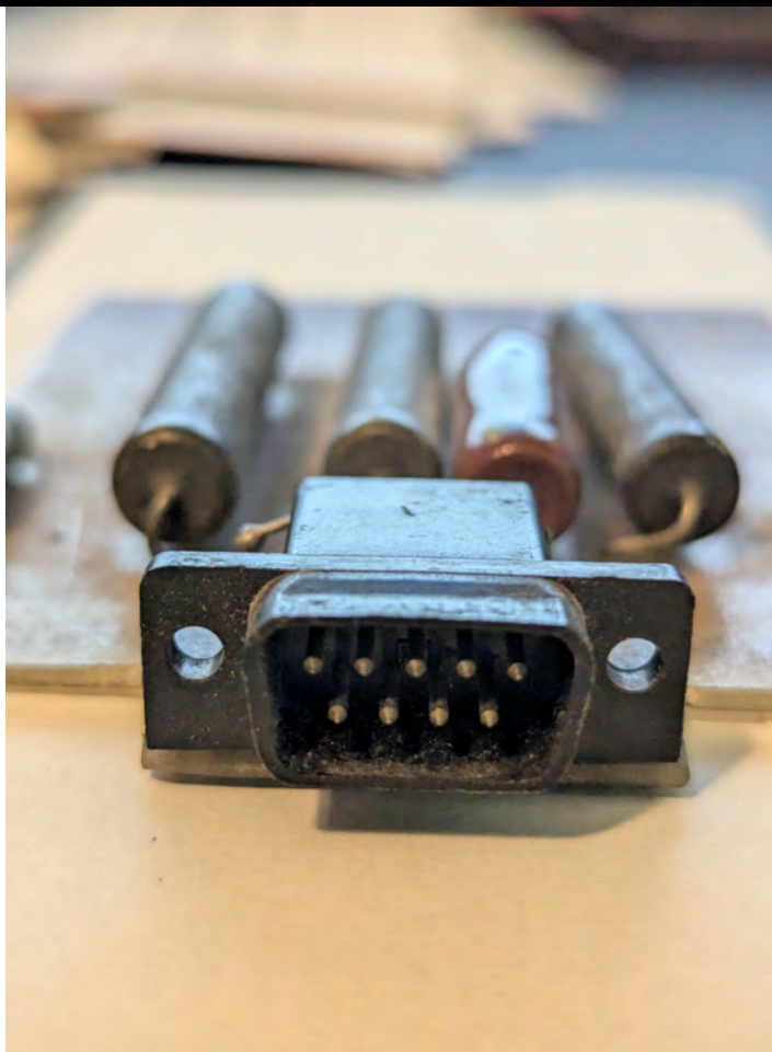
Figure 4 — DE-9 (DB-9) male connector at the board edge, face-on. Nine pins arranged in the standard 5-over-4 D-subminiature pattern. This is the same connector type and pinout as the ADAM console's power input.
