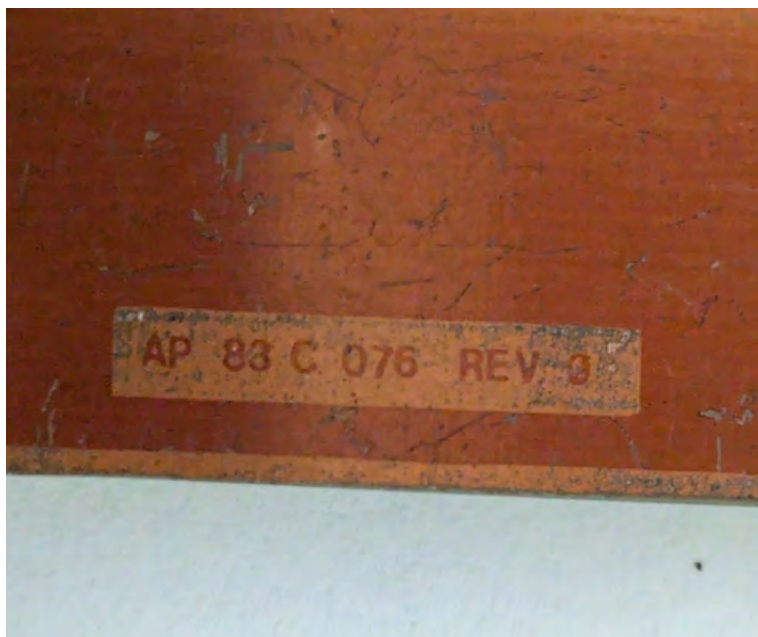
Figure 1 — Foil P/N sticker on the solder side. The label reads (rotated 90° from the photo): AP 83 C 076 REV 0. The "AP" prefix is a Coleco internal category code; "83" is the year, "C" the variant code, "076" the sequence, and "0" the initial revision.
