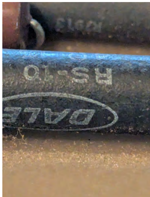
Figure 6 — R1 close-up showing the body silkscreen 4Ω 1% 10W 7038. The "7038" is a Dale internal lot/part-code suffix.
