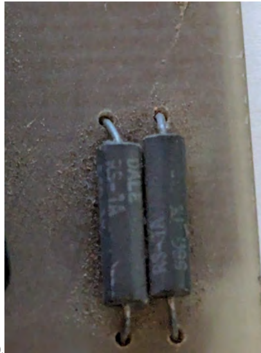
Figure 9 — Close-up of the two small vertically-mounted wirewound resistors at the right edge of the board (R6, R7). Dale brand markings and "RS" family identifiers are visible but the specific \Omega values are not yet legible.
